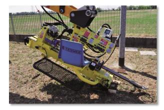
With its ability to be surface launched, pit launched, inverted and with set up angles of +/- 90 degrees and full 360 degree rotation this award winning drill is the ultimate machine for last mile fiber connections.
