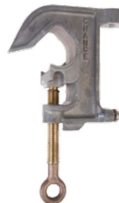
C6001743 Aluminum body, Smooth jaws, Bronze eyescrew with fine threads, Tapped for 5/8-11 UNC threaded ferrule
