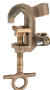
C6001959 Bronze body, Smooth jaws, Bronze T-handle/eyescrew with fine threads, Tapped for 5/8-11 UNC threaded ferrule
