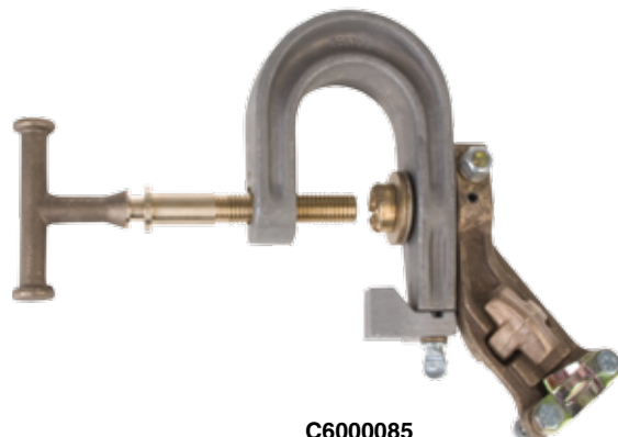
C6000085 Aluminum body and retainer, Bronze scrubber-type contact pads, Bronze T-handle with fine threads, Bronze pressure-type terminal
