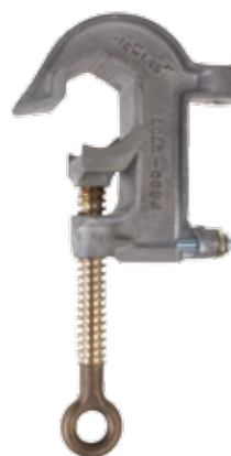
T6002708 Aluminum body, Serrated jaws, Bronze eyescrew with Acme threads, Tapped for 5/8-11 UNC threaded ferrule
