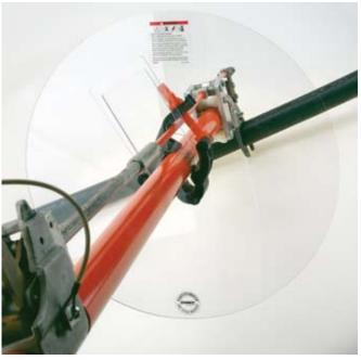
Tested per ASTM Standard F2522-05: Test Method for Determining the Protective Performance of a Shield Attached on Live Line Tools or on Racking Rods for Electrical Arc.
