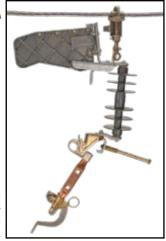
parallel with the permanent tap connection. After closing the blade of the tool, the permanent tap can be disconnected. The load can then be dropped or reconnected by operating the blade of the tool. It should never be closed into a fault or opened during a fault.
