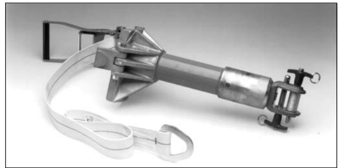
Dual-pin/single-roller set-up lets you rig the bracket for mounting on either side of the pole. So strap always rides on the roller, place roller on appropriate push-button pin.
