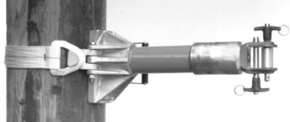
Dual-pin/single-roller set-up lets you rig the bracket for mounting on either side of the pole. So strap always rides on the roller, place roller on appropriate push-button pin.
