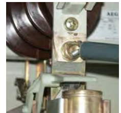
Testing with screwed-on V-shaped electrode
