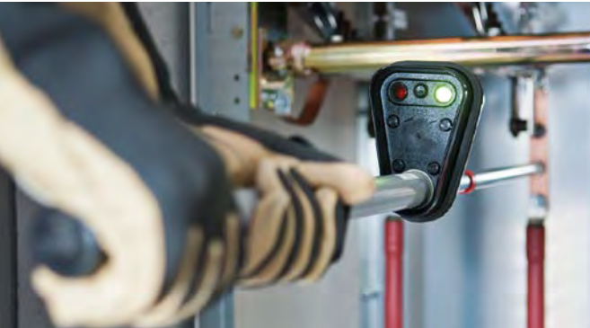
PHE voltage detector with visual indication
