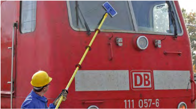
Insulating stick kit used for cleaning the windscreen of an electric locomotive
