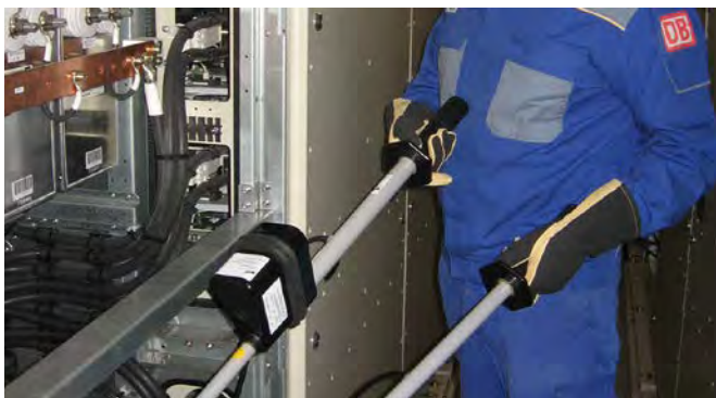
PHE/G II d.c. voltage detector for d.c. links (ICE power car)
