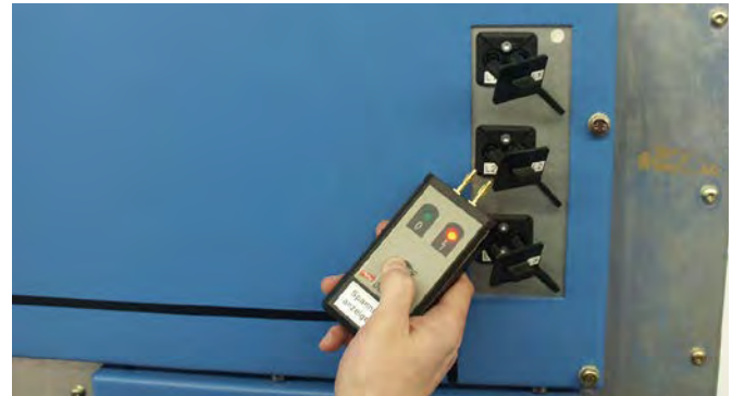
Self-test of a DEHNcap/A voltage indicator
