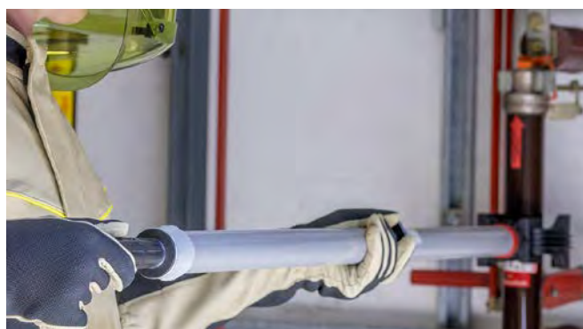
SZ fuse tongs for inserting and removing HH fuses
